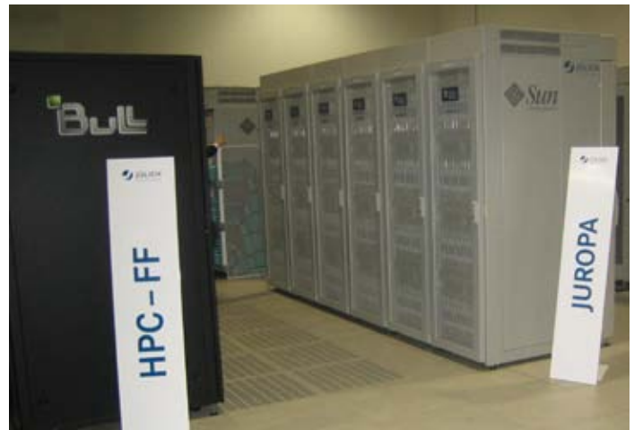
JUROPA and the fusion machine HPC-FF together provide up to 308 Teraflops peak performance
