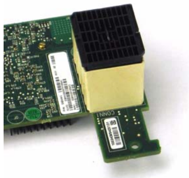
Figure 7: Protective Cover in Place
