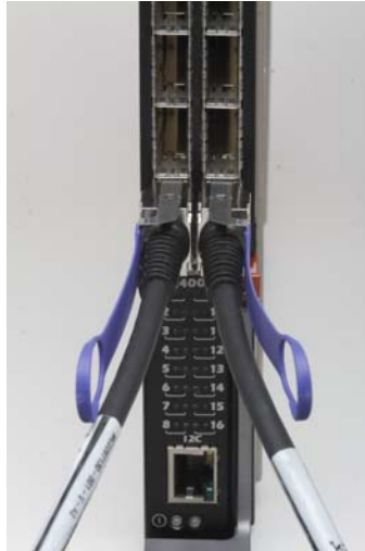
Figure 6: Belly to Belly Cable Insertion
