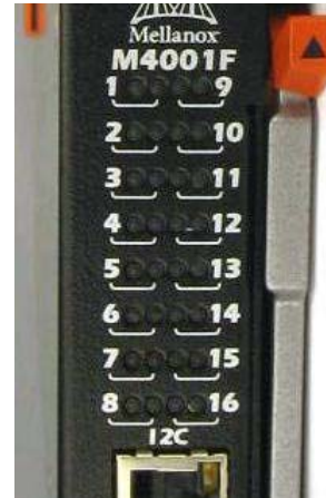
Figure 2: Physical and Logical Link Indication LEDs
