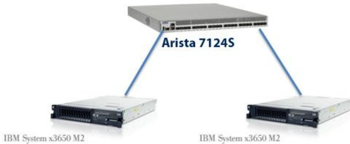
**Figure 1: Test configuration**
