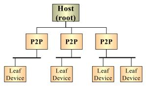
As mentioned the PCI architecture utilizes a flat unified memory architecture and use of PCI to PCI bridges for scaling means that systems must be constructed using a hierarchical tree structure. The PCI architecture requires this as a PCI to PCI bridge has a primary (or upstream) bus and a secondary (or downstream) bus. At the top of a PCI system there is a single master (or root) host PCI segments and at leaf PCI segments at endpoints. Standard PCI boot software understands this hierar-
