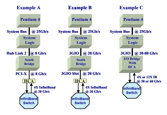
Example B shows how PCI-Express can be used to upgrade the bandwidth of both the interconnect between system logic and the south bridge, as well as, the PCI slot. In the implementation shown PCI-Express can be scaled to support the 20 Gb/sec InfiniBand requires in both locations. This implementation enables InfiniBand 4X bandwidth (20Gb/s) from a Pentium 4 processor, across the I/O subsystem and onto the InfiniBand fabric.
