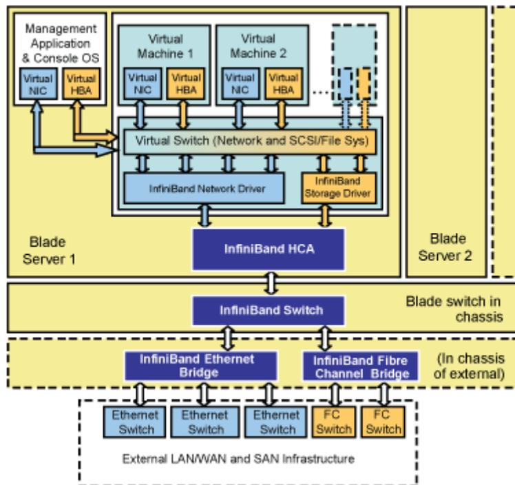
Figure 5: Software-based I/O Virtualization with InfiniBand adapters and gateways
