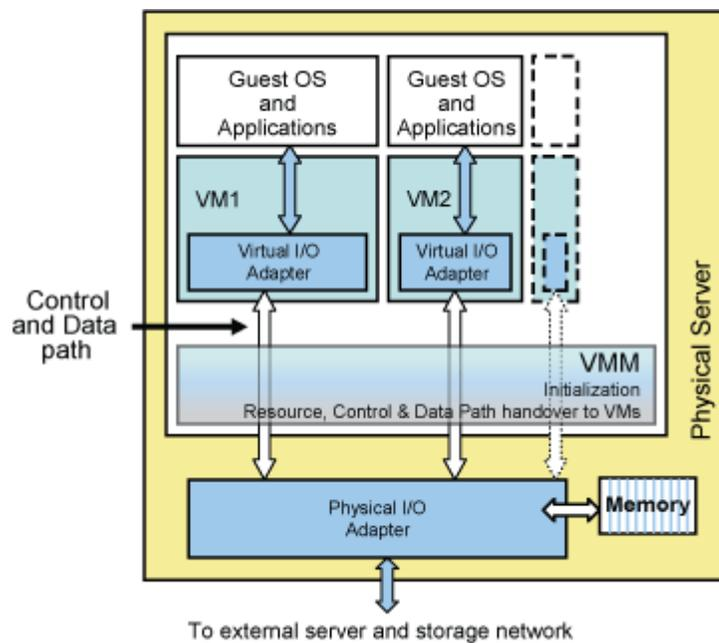
**Figure 10: Hardware-based I/O Virtualization**
