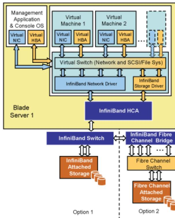
Figure 6: Use of InfiniBand for Server-to-Server and SAN connectivity functions
