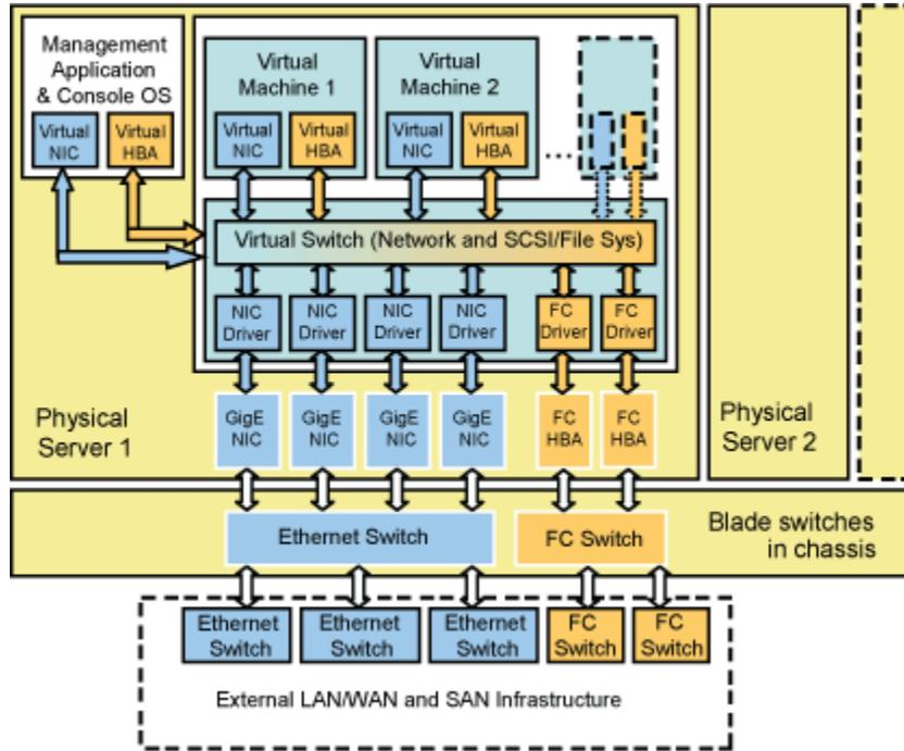
Figure 4: Software-based I/O Virtualization with multiple GigE NIC and FC adapters
