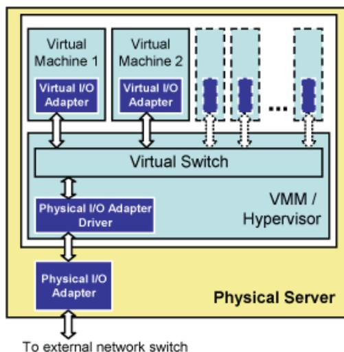
Figure 2: Software-based I/O Virtualization
