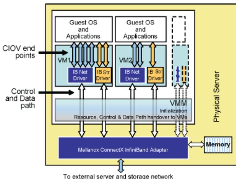
**Figure 11: Hardware-based I/O Virtualization using InfiniBand and CIOV**
