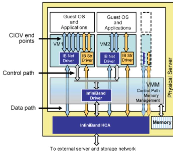
Figure 8: Mellanox InfiniBand and CIOV with Native I/O Virtualization
