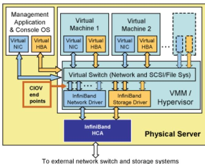
Figure 3: Mellanox CIOV with Software-based I/O Virtualization
