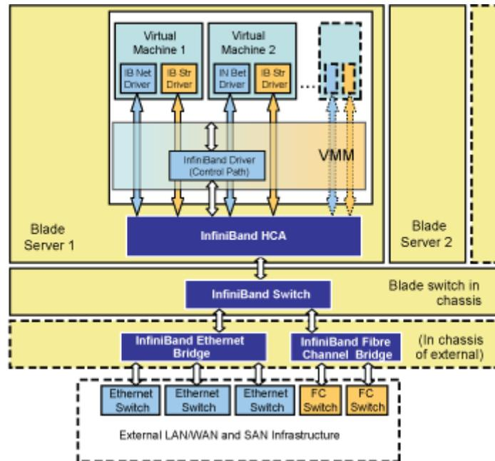
Figure 9: Use of InfiniBand in a Native I/O Virtualization Deployment Scenario
