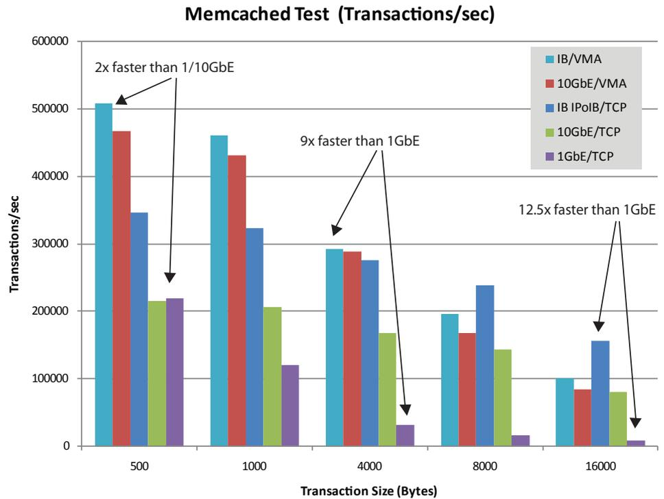
It can be seen that VMA with InfiniBand provides the highest transaction per seconds compared to other solutions. Mellanox 10GbE with VMA outperforms traditional 10GbE infrastructures by 2X on smaller packets.
