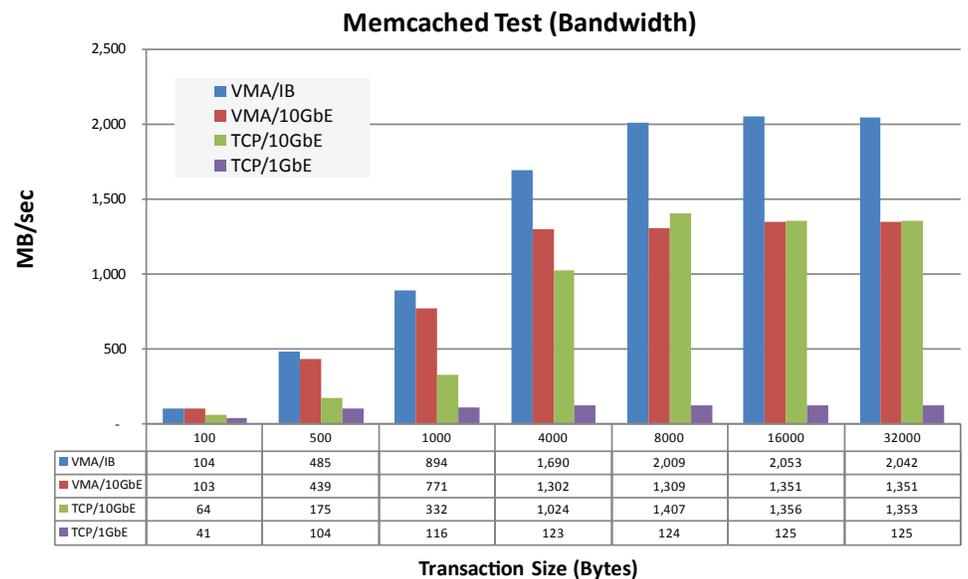
Highest bandwidth was achieved with InfiniBand infrastructure and VMA compared to 10GbE and TCP.
