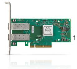
Notes: All tall-bracket adapters are shipped with the tall bracket mounted and a short bracket as an accessory.
