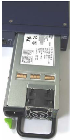
Figure 15: Power Supply Unit Extraction
