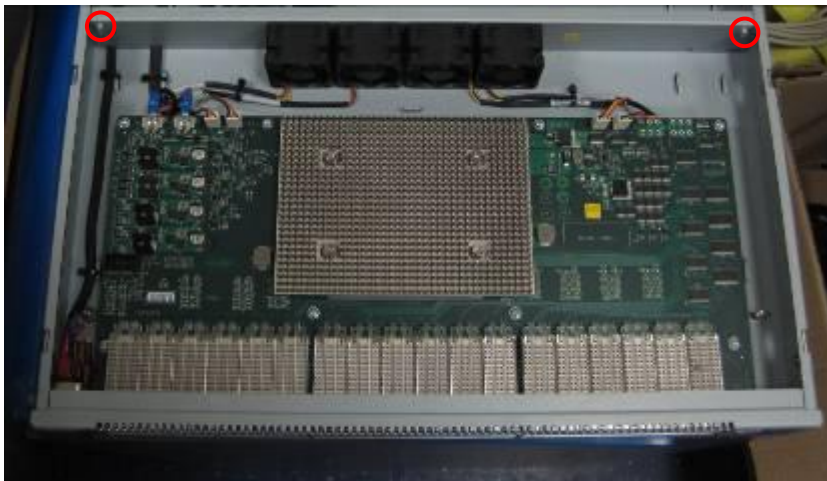
Figure 6 Fan Top Side Screw Locations
