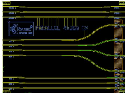
Figure 2(b): Mask layout of SiP Rx with Ge Detectors
