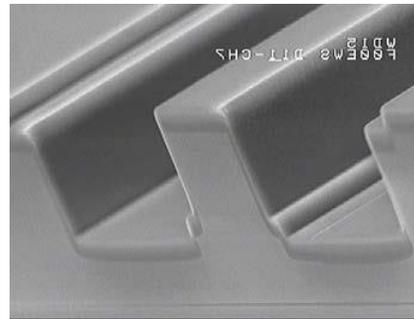
Figure 1(b) SEM view of mode transformer
