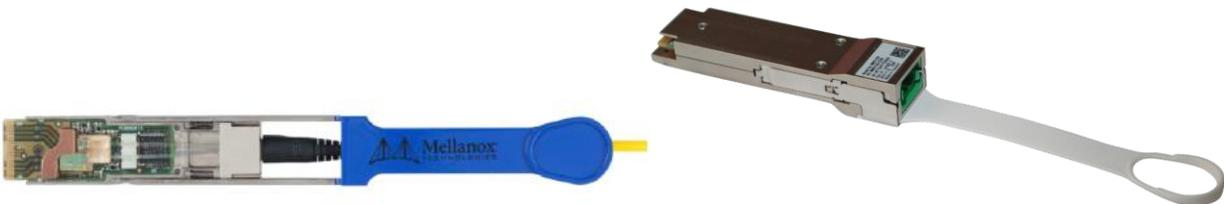
Figures 2 (c): Top removed from a 100 Gb/s SiP transceiver; a fully packaged QSFP28 transceiver.
