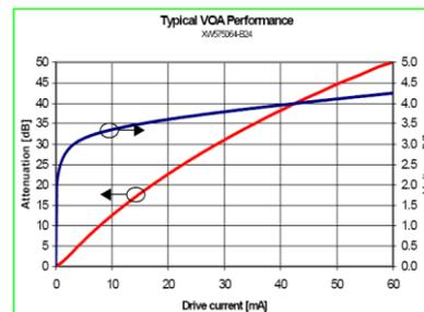
Figure 1(d). Measured VOA performance
