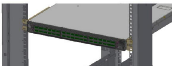
Figure 6: Sliding the Blades in the Rails
