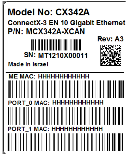
Figure 3: MCX342A-XCAN Board Label
