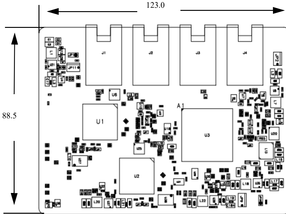
Figure 3: Mechanical Drawing of the MCX349A-XCCN Mezzanine Card
