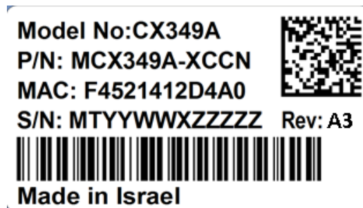
Figure 4: MCX349A-XCCN Board Label (Example only - see Note)
