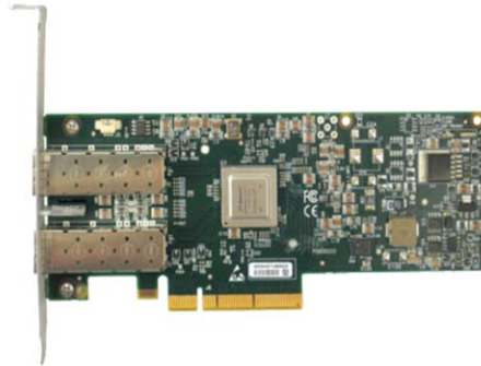
FIGURE 2: MELLANOX CONNECTX-2 EN WITH ROE NICS (DUAL SFP+ CARD SHOWN)
