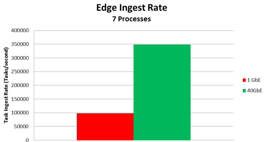
Figure 7: Edge Ingest Test Results
