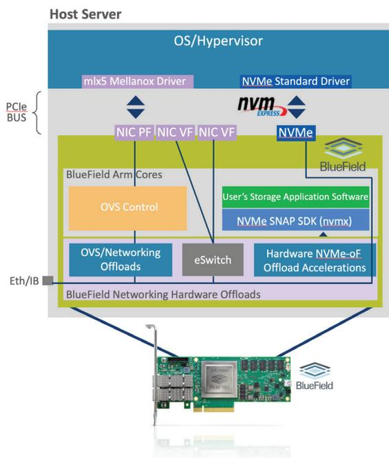
**Figure 5:** BlueField SmartNIC with NVMe SNAP serves as a smart network adapter for both storage and network virtualization simultaneously
