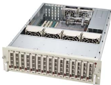
Figure 5. SC933T Native InfiniBand Storage Platform and Measured Performance Advantage vs Fibre Channel
