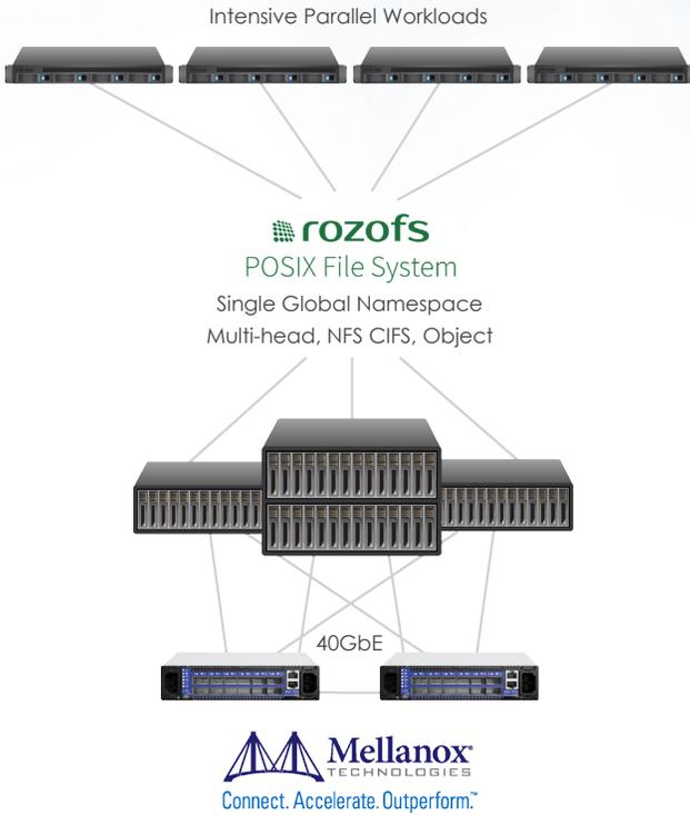
To select the right networking devices, Rozo Systems completed a successful trial with Mellanox’s 40GbE end-to-end solution (SX1012 Ethernet switch and ConnectX®-3 Pro network adapter cards). The results demonstrate that Mellanox Ethernet products are able to deliver the performance required by Rozo’s high performance cluster file system.
