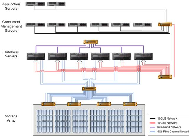
During the POC, a set of invoices was stored and processed twice: once using each of the InfiniBand 40Gb/s and 10GbE configurations. The results show that when InfiniBand was used, the number of invoices processed per second was higher by 63 percent compared to the configuration that was based on 10GbE.
