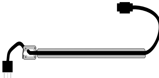
Figure 18: Put the Cord Through the Switch Slide Before Screwing it to the Switch
