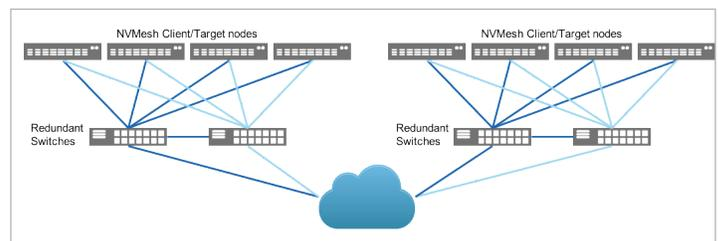
The Mellanox-Excelero solution was designed to let applications enjoy full performance, capacity and processing power of underlying servers and storage. Leveraging the NVMe RDMA technology, the solution adds a mere 5µs latency over local NVMe drive latency, allowing customers to leverage full performance of their hardware at data center scale. The solution enables customers to achieve higher performance levels than proprietary all-flash-arrays at a much lower \$/IOP, or \$/GB/s.
