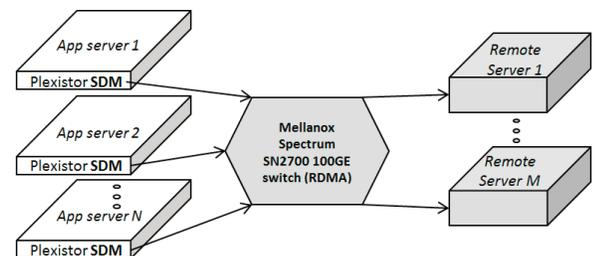
In recent testing, N single-socket E5-2667v3 application servers, running CentOS 7.2, were each installed with Plexistor SDM<sup>1</sup> software and a
