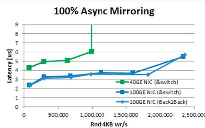
Using the synthetic FIO benchmark<sup>2</sup>, latency was measured as a function of throughput for the most demanding workload: 100% random Write accesses. Each Write access was measured end-to-end, i.e., from before the user space application triggered the Write system call, via the context switches, until after it completed, resulting in a persistent local copy and a volatile confirmed/unconfirmed second copy of the data and metadata on the remote node.
