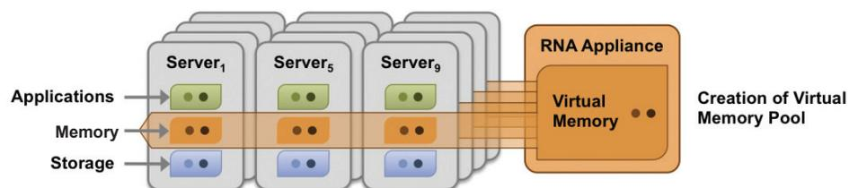
Server clusters already rely on remote direct memory access (RDMA) to divide application tasks among CPUs and servers, and RNA's MVP builds on RDMA to provide the fastest possible memory access for all servers in the cluster at any time. In fact, MVP can also scale to very high bandwidth by incorporating portions of each server's memory as part of the virtualized pool. Integrating memory from multiple servers also makes it very easy to scale up the
