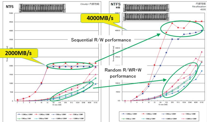
These performance levels are higher than the 4K 12bit 4:4:4 60p Uncompressed Video rate and well match to 25GbE bandwidth speeds. In the near future we plan to increase performance more to be balance with Infiniband 56Gbps speed. These performance levels will enable us to support 8K 10bit 4:2:2 60p Uncompressed Video.
